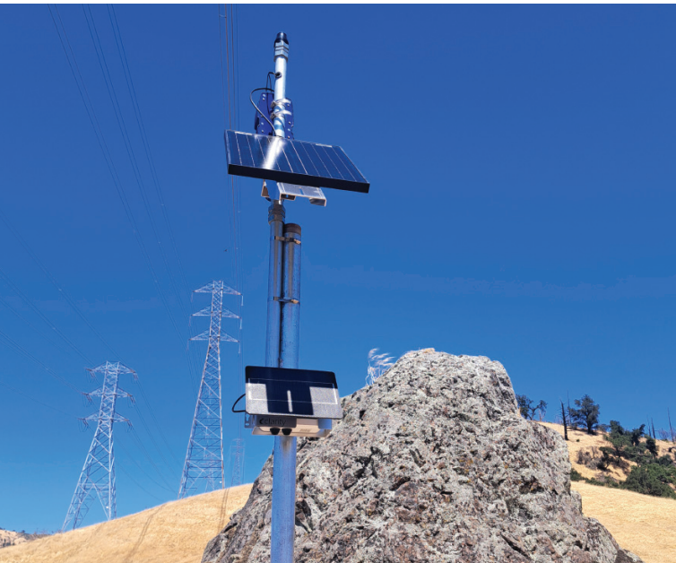
Left: A Clarity Node air quality sensor (bottom) and a N5 sensor for wildfire detection (top) at Modini Preserve. Photo: Ryan Ferrell. Right: Arrows show locations and viewscape for the ALERTCalifornia network, which more than doubled its number of camera sensors between 2019 and 2023.
